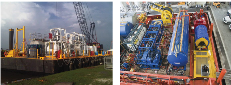
FIGURE 3.4 Two BPWS Integrated Systems installed on the D&L Salvage spud barge The Splash (left) and four BPWS Integrated Systems installed on Edison Chouest platform supply vessel ELLA G (right).
